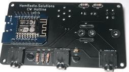
Install the speaker leads into pads marked SP1. If the speaker has a connector on the end of the leads, remove it and strip the insulation. The red wire should go to the square hole. Solder on the other side. Use the small square of double sided foam tape to stick the speaker to the PCB above the circle.
